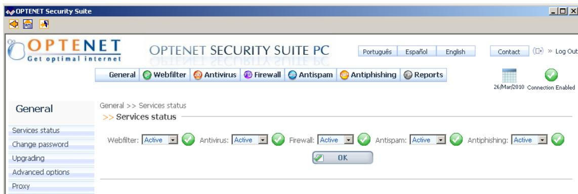
There is a combo box enabling independently the activation/deactivation of each service. An icon indicates whether the service is currently active or not. If a service is not active, the configured filtering restrictions will not be applied.
